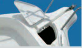
**630 Commander.**A bow roller, recessed anchor line channel, in-line cleat and anchor locker are top quality features on the 630 series.
